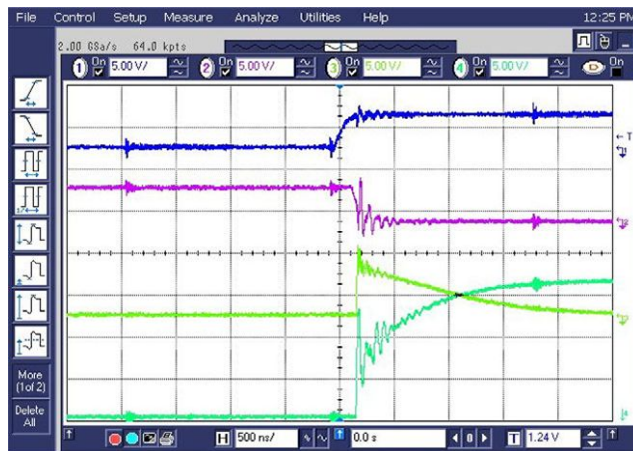
Fig. 13 - Preload (Purple) and Voltage at the Gate (Bright Blue)
