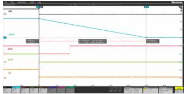
Fig. 7 - Shut Down by EN ( I_{OUT} = 2\text{ A} , C_{OUT} = 10\text{ mF} )
