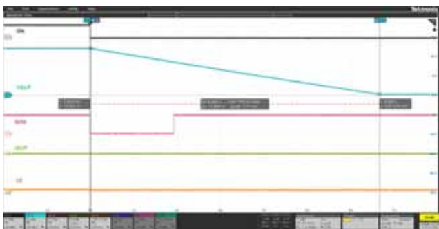
Fig. 6 - Shut Down by EN ( I_{OUT} = 0\text{ A} , C_{OUT} = 10\text{ mF} )
