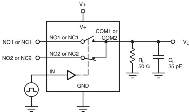
$C_L$  (includes fixture and stray capacitance)
