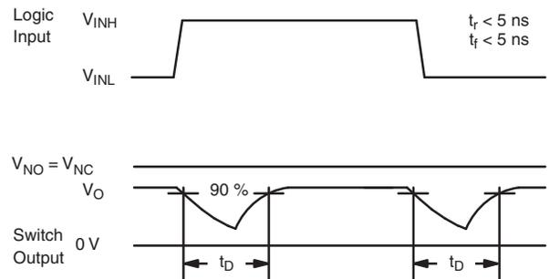
Fig. 2 - Break-Before-Make Interval
