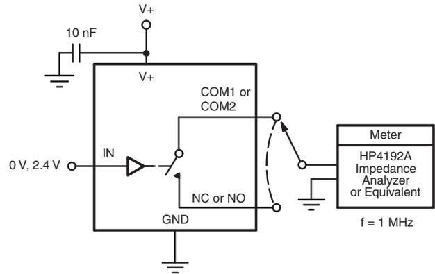
Fig. 5 - Channel Off/On Capacitance
