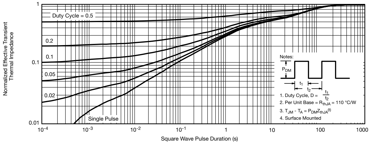
Normalized Thermal Transient Impedance, Junction-to-Ambient
