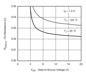
On-Resistance vs. Gate-to-Source Voltage
