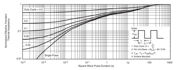
Normalized Thermal Transient Impedance, Junction-to-Ambient
