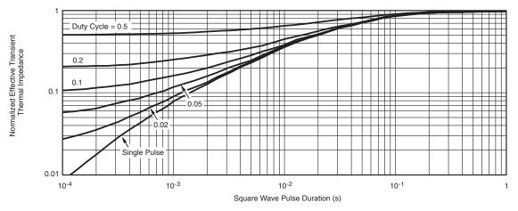
Normalized Thermal Transient Impedance, Junction-to-Foot
