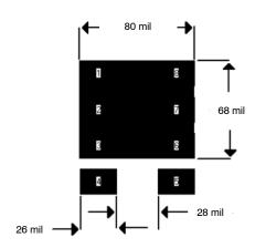
FIGURE 2. Footprint With Copper Spreading
