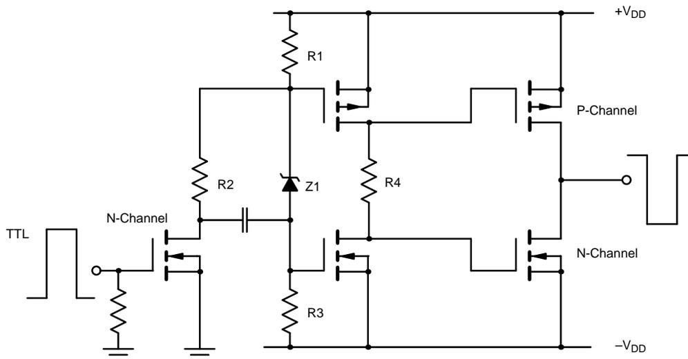
**FIGURE 6.** High-Voltage Complementary Pair Driven by Logic-Compatible MOSFET
