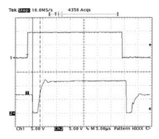
FIGURE 6. Si4720CY/Schottky Diode Switching
