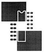
SO-16 with Heat Spreading Pads. Pad Dimension 0.320 x 0.260
