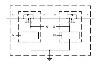
FIGURE 2. Discrete Circuit and Si4720CY Equivalent Circuit
