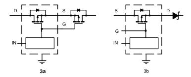
FIGURE 3. Si4720CY Switch, 1/2 Si4720cy with MOSFET, 1/2 Si4720CY with Schottky
