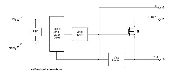
FIGURE 1. Si4720CY Functional Block Diagram
