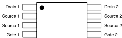
Figure 3. Pinouts for Dual-Die TSSOP
