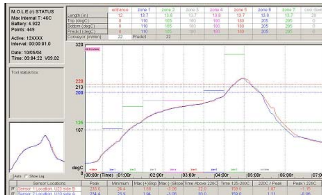
Figure 3: LRSS profile for lead (Pb)-free solder paste Peak temperature: 235 °C Time above 220 °C: 32 seconds Soak time (120-200 °C): 159 seconds
