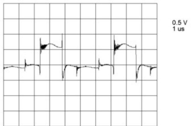
Resistor/Diode clamped Synchronous Rectifier Drains - TP21 or TP22 measured with respect to ground (TP14).
