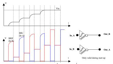
Figure 7. Rise of Vin and SRL' and SRH' signals during start-up.
