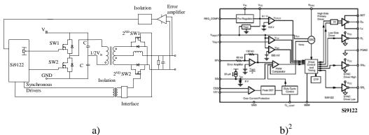
Figure 1. Block diagram of half-bridge topology and Si9122 IC.
