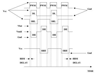
Figure 4. BBM timing diagrams.
