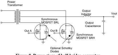
Figure 8. Power stage of half-bridge converter
