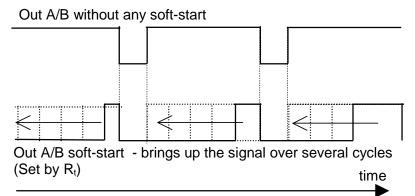
Figure 10. Soft-start of the output drivers.
