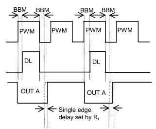
Figure 11. Single edge delay set by an external resistor.
