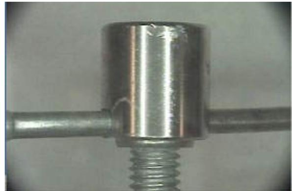
Figure 9c. C-clamp head with socket adaptor
