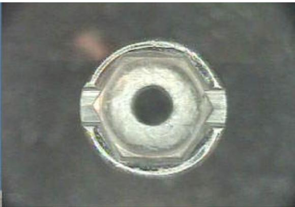
Figure 3b. Socket Adaptor Bottom View
