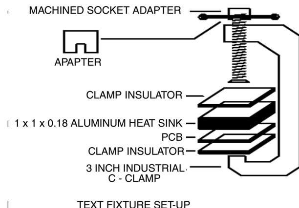
Figure 2. Mechanical test fixture
