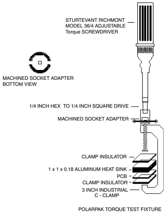
Figure 9a. Complete clamping and torque setting arrangement
