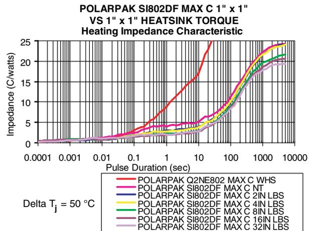
Figure 10. Transient thermal characteristics at different torque values
