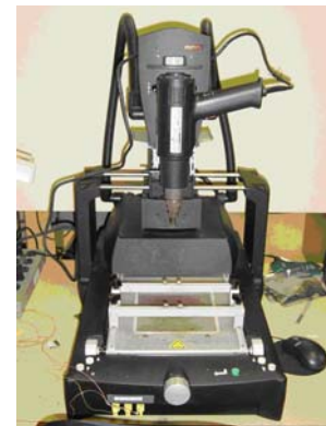
Figure 7. Mechanical fixture to hold the heat gun
