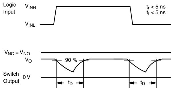
Fig. 2 - Break-Before-Make Interval
