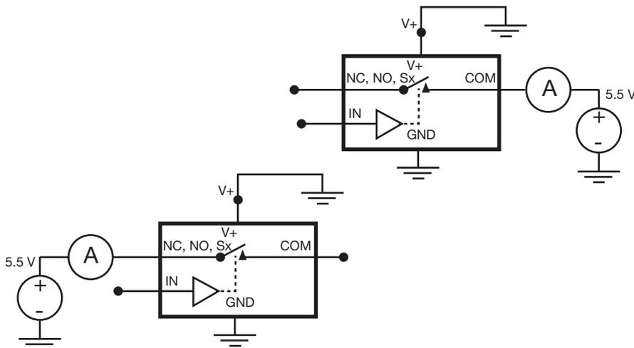
Fig. 6 - Source / Drain Power Down Leakage
