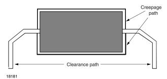
Fig. 1 - Isolation Creepage/Clearance Path Along the Body
