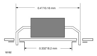
Fig. 2 - Isolation Creepage/Clearance Path after Mounting on a Board (Side View)
