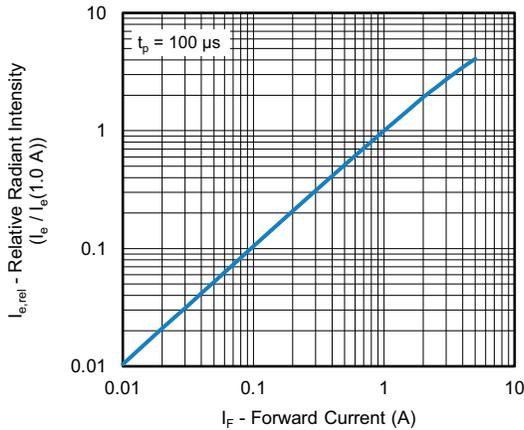
Fig. 5 - Relative Radiant Intensity vs. Forward Current
