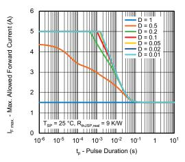
Fig. 9 - Max. Allowed Forward Current vs. Pulse Duration
