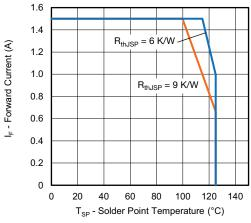
Fig. 2 - Forward Current Limit vs. Solder Point Temperature
