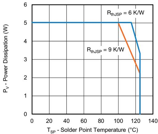
Fig. 1 - Power Dissipation Limit vs. Solder Point Temperature
