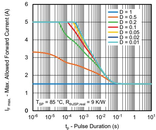
Fig. 10 - Max. Allowed Forward Current vs. Pulse Duration
