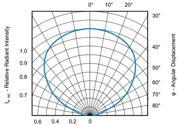
Fig. 8 - Relative Radiant Intensity vs. Angular Displacement
