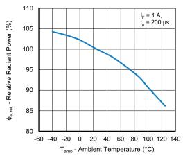
Fig. 6 - Relative Radiant Power vs. Ambient Temperature
