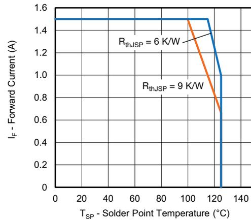
Fig. 2 - Forward Current Limit vs. Solder Point Temperature
