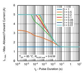
Fig. 10 - Max. Allowed Forward Current vs. Pulse Duration
