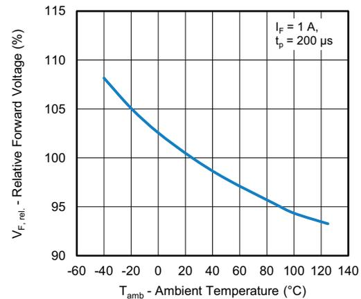
Fig. 4 - Relative Forward Voltage vs. Ambient Temperature
