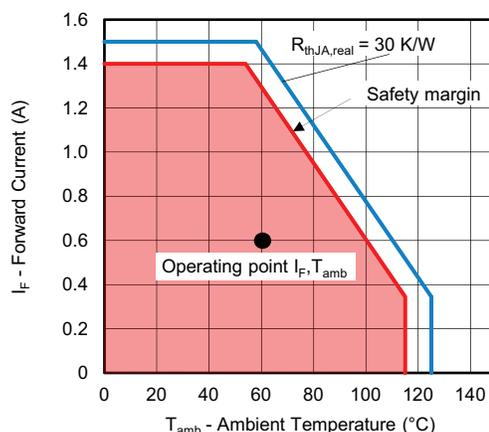
Fig. 26 - Derating Diagram With Safety Margin
