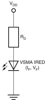
Fig. 5 - Example Circuit With a Current Limiting Resistor
