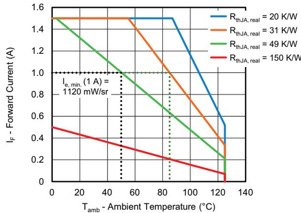
Fig. 28 - Derating Diagram Based on  $R_{thJA, \text{real}}$
