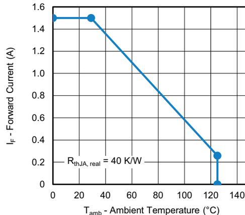
Fig. 27 - DC Derating Diagram With  $R_{thJA, real} = 40 \text{ K/W}$
