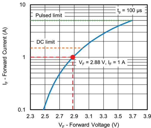
Fig. 7 - DC Operating Point Example for the VSMA1094250X02
