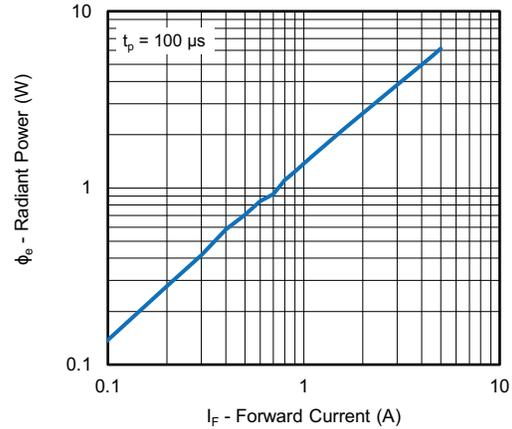
Fig. 3 - Radiant Power vs. Forward Current for the VSMA1094250X02
