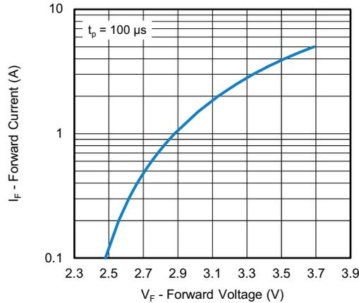
Fig. 4 - Forward Current vs. Forward Voltage for the VSMA1094250X02
