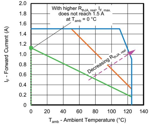
Fig. 21 - The Effect of Higher  $R_{thJA, real}$
