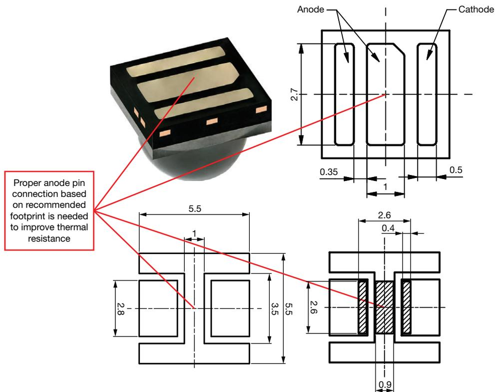
Fig. 25 - Anode Pin Connection in the Middle of the VSMA1094250X02
