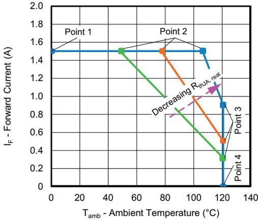
Fig. 20 - Four Important Points on DC Derating Diagram
