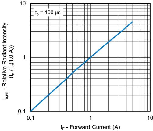
Fig. 2 - Relative Radiant Intensity vs. Forward Current for the VSMA1094250X02
