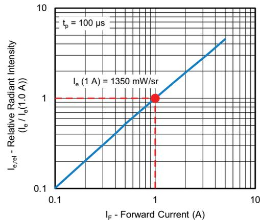
Fig. 8 - Relative Radiant Intensity vs. Forward Current for the VSMA1094250X02
