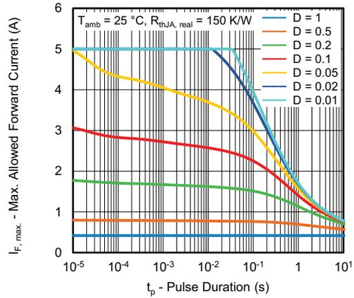
Fig. 35 - Pulse Derating Diagram Based on FR4 PCB at 25 °C
