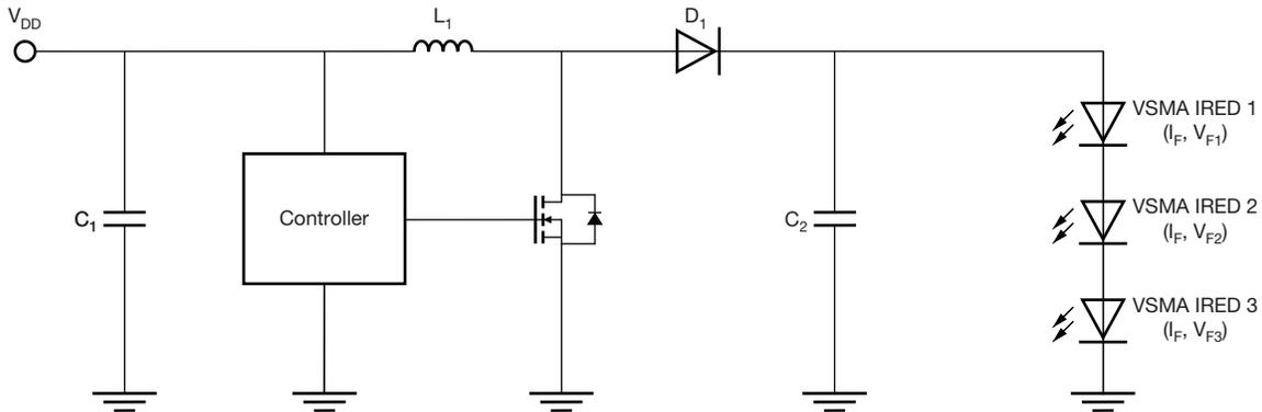
Fig. 11 - Example Circuit With a PWM-Controlled Boost Regulator
