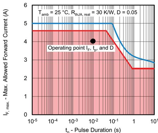
Fig. 40 - Pulse Derating Diagram With Safety Margin
