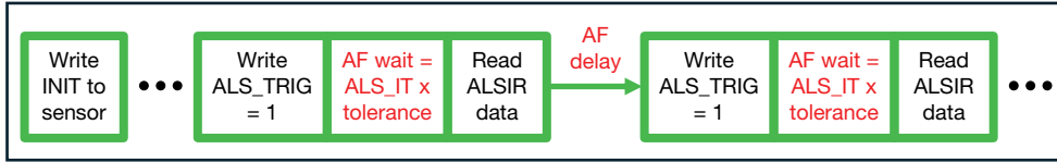
VEML4031X00 timing diagram for active force mode (AF mode)
