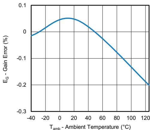
Fig. 7 - Gain Error vs. Ambient Temperature
