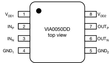
Fig. 2 - VIA0050DD Package
