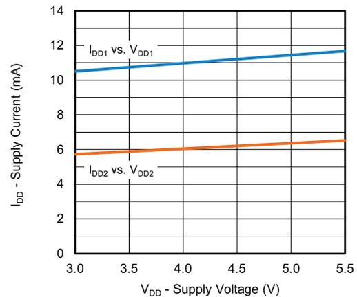
Fig. 18 - Supply Current vs. Supply Voltage
