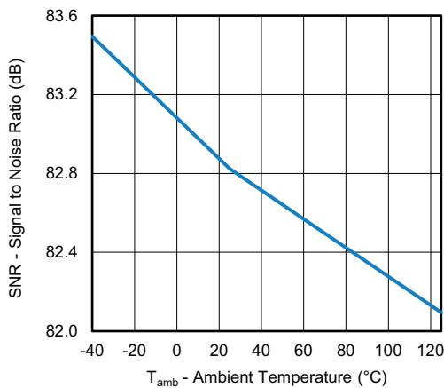
Fig. 13 - Signal to Noise Ratio vs. Ambient Temperature
