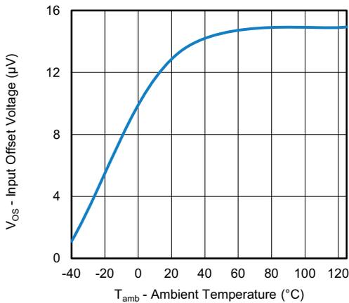
Fig. 4 - Input Offset Voltage vs. Ambient Temperature
