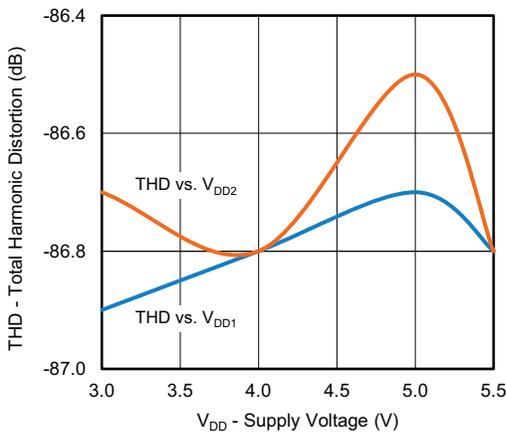
Fig. 9 - Total Harmonic Distortion vs. Supply Voltage
