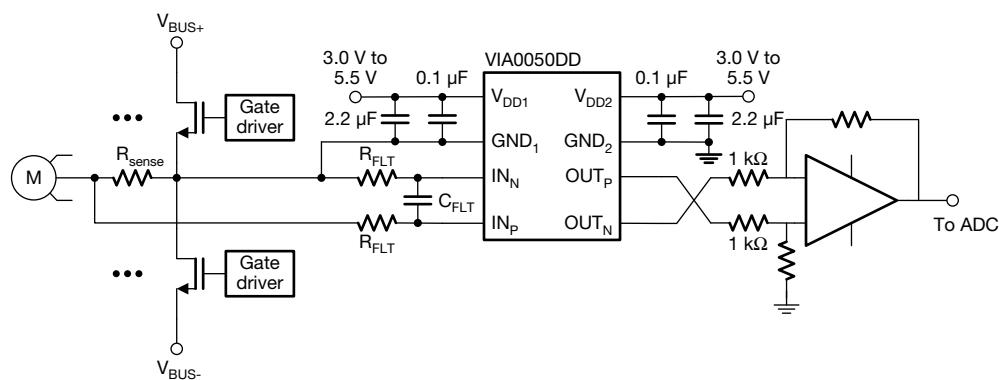
Fig. 25 - Typical Application Circuit in Phase Current Sensing
