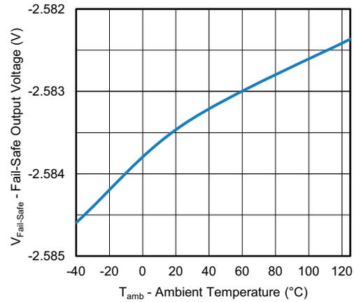
Fig. 16 - Fail-Safe Output Voltage vs. Ambient Temperature
