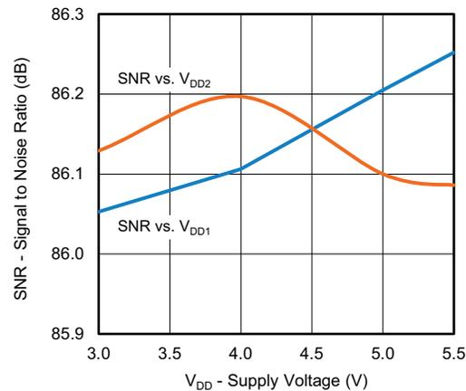
Fig. 12 - Signal to Noise Ratio vs. Supply Voltage
