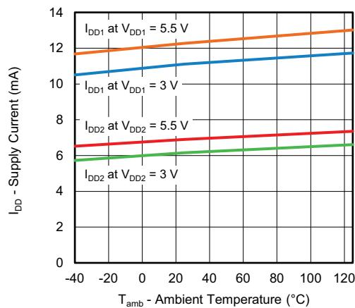
Fig. 20 - Supply Current vs. Ambient Temperature
