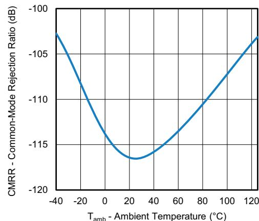
Fig. 5 - Common-Mode Rejection Ratio vs. Ambient Temperature
