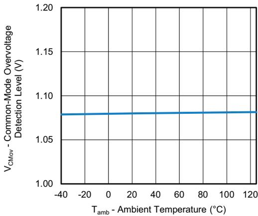
Fig. 3 - Common-Mode Overvoltage Detection Level vs. Ambient Temperature
