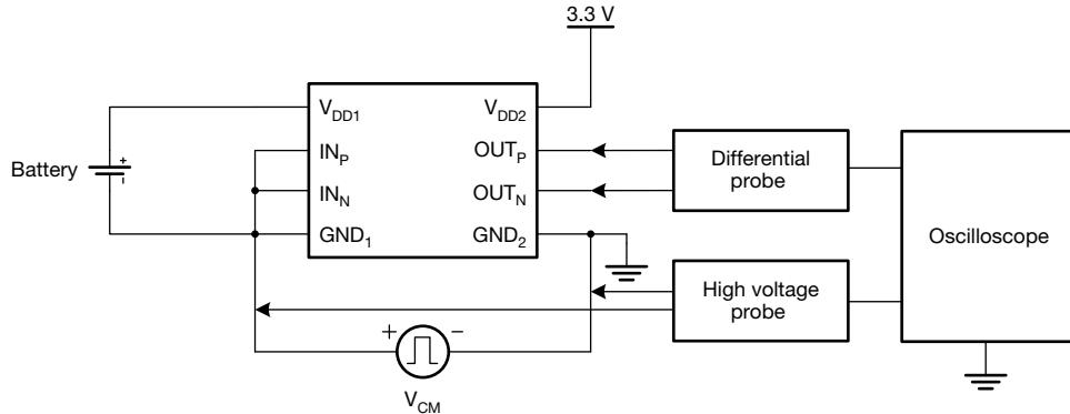
Fig. 22 - Common-Mode Transient Immunity Test Circuit
