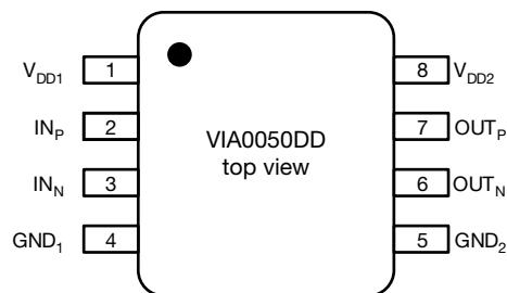
Fig. 2 - VIA0050DD Package
