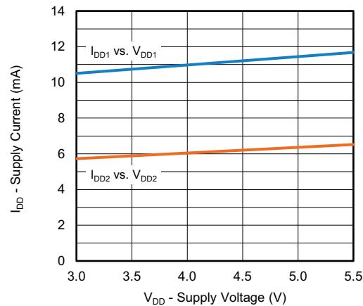
Fig. 18 - Supply Current vs. Supply Voltage
