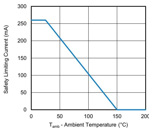
Fig. 23 - VIA0050DD Thermal Derating Curve, Dependence of Safety Limiting Values With Case Temperature per DIN VOE V0884-11
