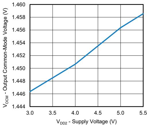
Fig. 14 - Output Common-Mode Voltage vs. Supply Voltage
