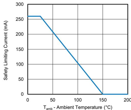
Fig. 23 - VIA0050DD Thermal Derating Curve, Dependence of Safety Limiting Values With Case Temperature per DIN VDE 0884-11
