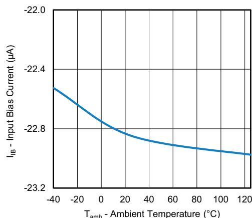
Fig. 6 - Input Bias Current vs. Ambient Temperature
