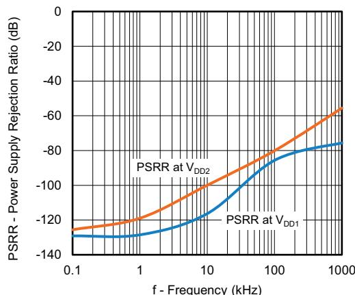
Fig. 19 - Power Supply Rejection Ratio vs. Ripple Frequency
