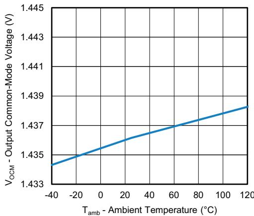
Fig. 15 - Output Common-Mode Voltage vs. Ambient Temperature
