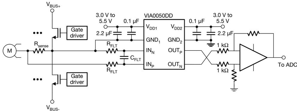
Fig. 25 - Typical Application Circuit in Phase Current Sensing
