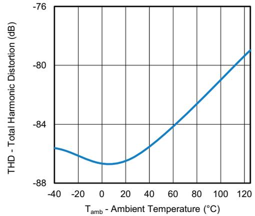
Fig. 10 - Total Harmonic Distortion vs. Ambient Temperature
