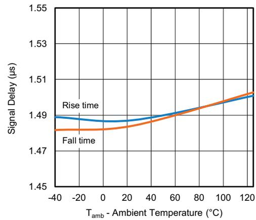
Fig. 17 - Signal Delay vs. Ambient Temperature
