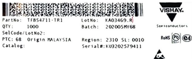
Fig. 2 - 2D Bar Code Label for a Lead (Pb)-Free Device Made in Malaysia, Equivalent to That Shown in Fig. 1
