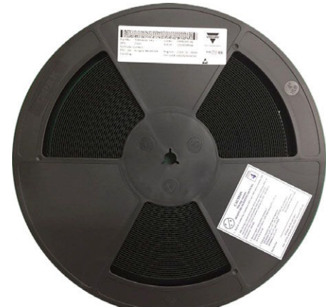
Fig. 13 - 330 mm Reel With Labels (Malaysia), no Labels on the Rear, Lead (Pb)-Free Marking is on the Bar Code
