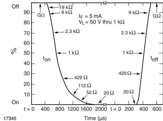
Fig. 1 - Dynamic Switching Resistance
