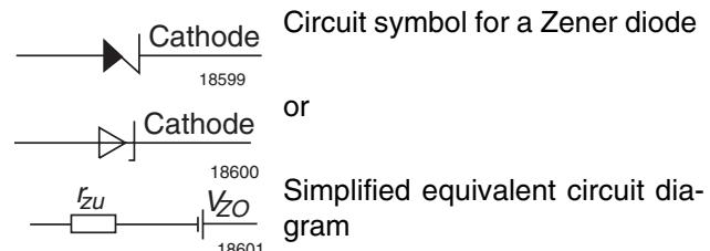
$V_{ZO}$  is the breakdown voltage, extrapolated for  $I_Z = 0$ .
