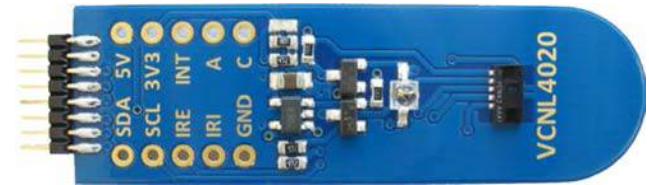
Fig. 6 - VCNL4020 Sensor Board
