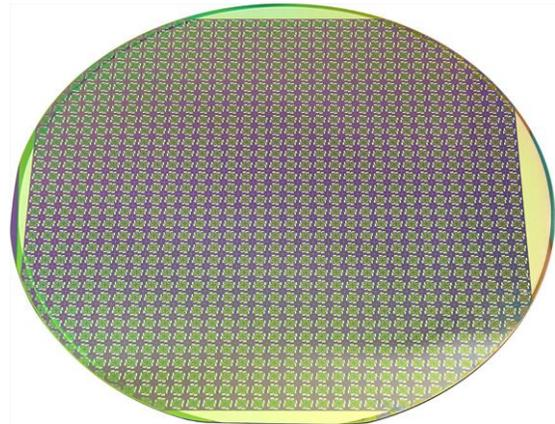
Fig. 4 - Nonsingulated Wafer
