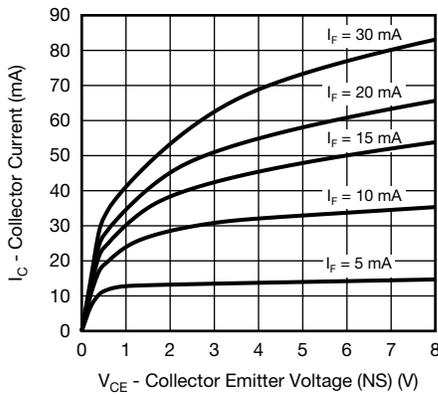
Fig. 2 - Collector Current vs. Collector Emitter Voltage (non-saturated)
