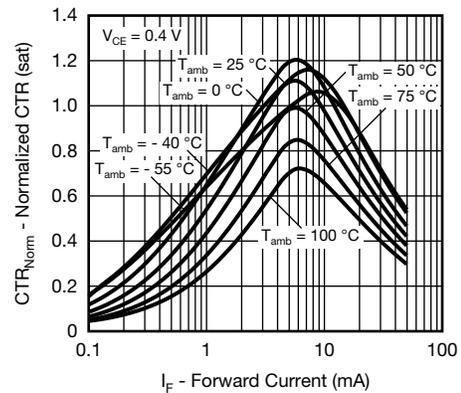
Fig. 5 - Normalized CTR vs. Forward Current (saturated)
