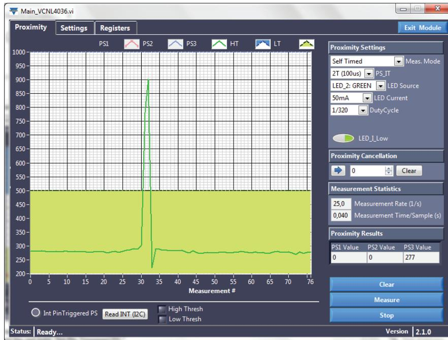
Fig. 25 - Just One Measurement Does Not Cause an Interrupt
