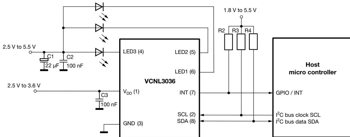
Fig. 3 - Circuitry With Two Separate Power Supply Sources
