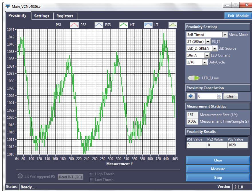
Fig. 29 - HRM Pulses Measured With the VCNL3036 Sensor Board
