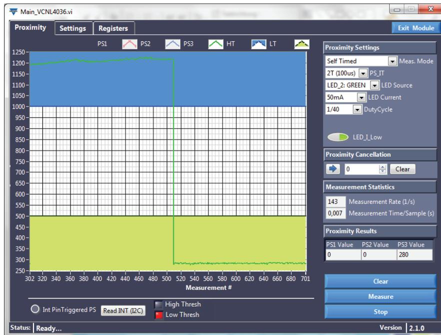
Fig. 26 - Finger Removed Again, Measured Counts Fall Back to the 300 Offset Counts
