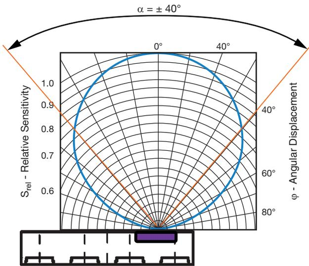
Fig. 6 - Proposed Angle of Relative Radiant Sensitivity
