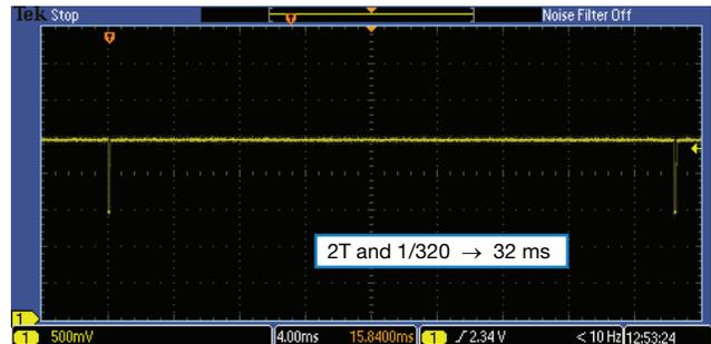
Fig. 14 - Proximity Measurements With PS\_Duty = 1/320
