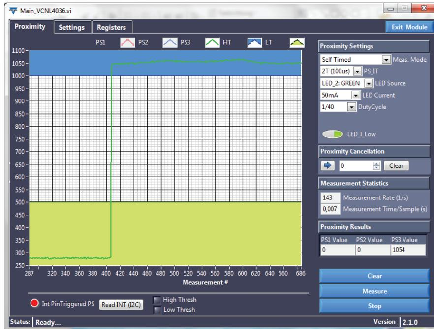
Fig. 23 - Upper and Lower Threshold Set and Finger Placed at Small Plastic Cover
