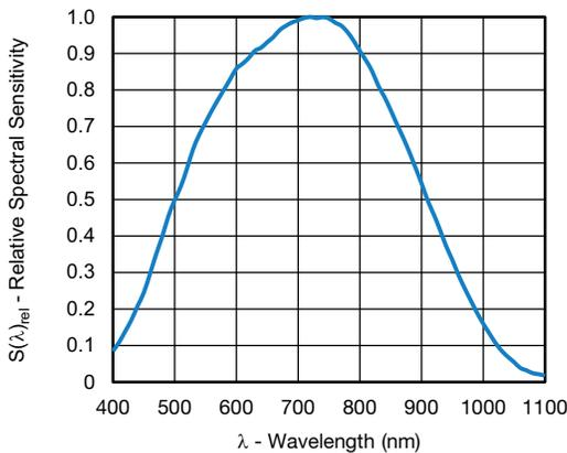
Fig. 9 - Normalized Spectral Response
