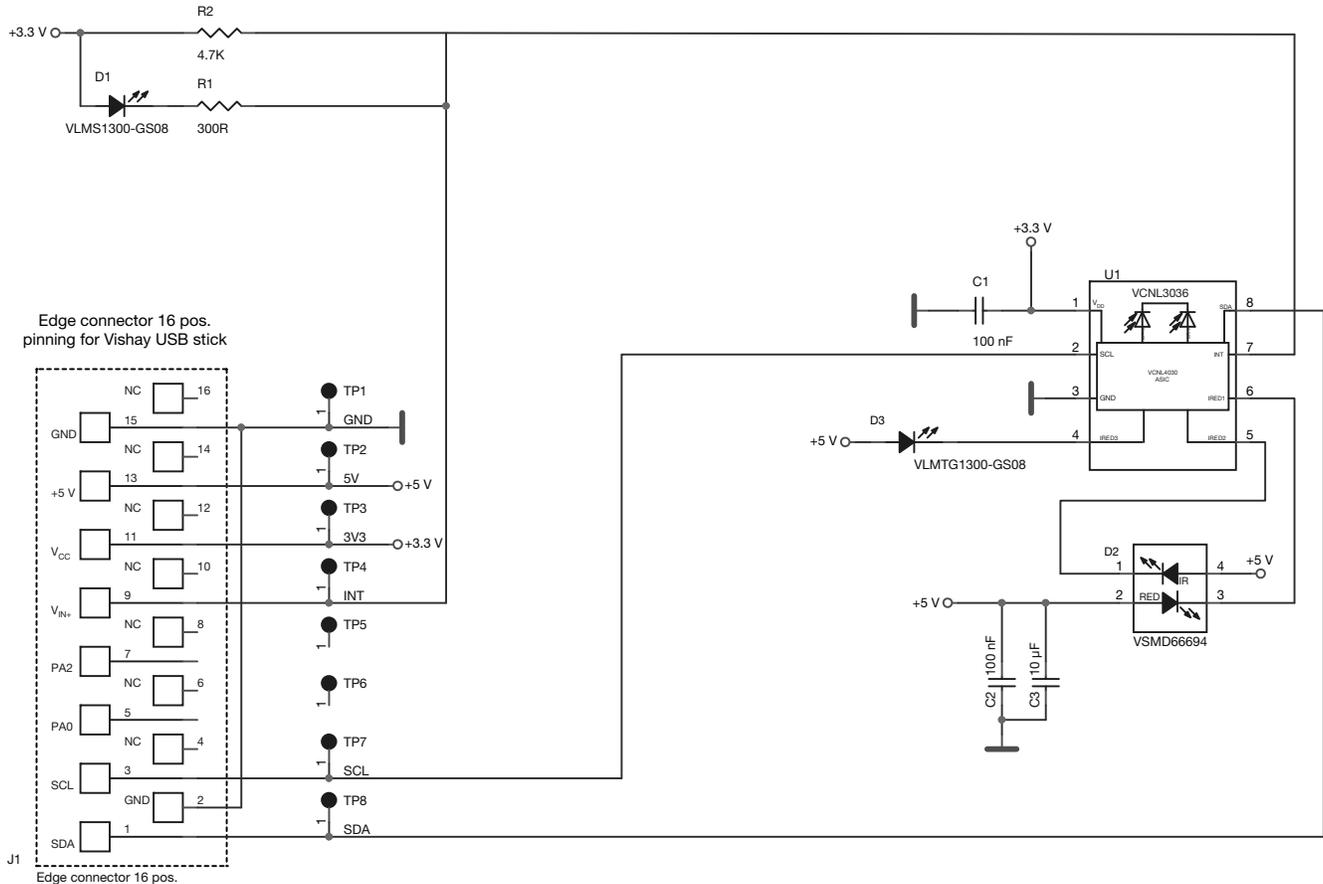
Fig. 38 - VCNL3036 Sensor Board Circuit Diagram
