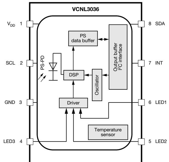
Fig. 2 - VCNL3036 Detailed Block Diagram
