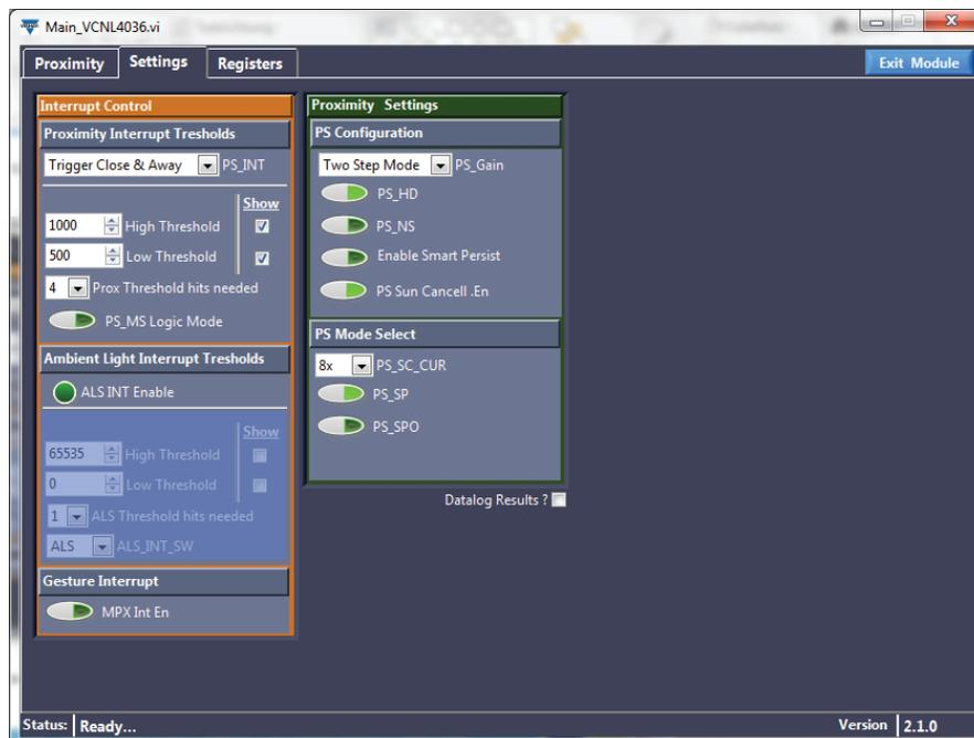
Fig. 24 - Upper and Lower Threshold Set and Four Hits Programmed
