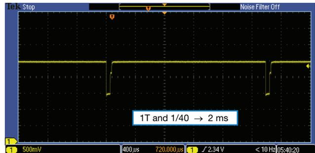
Fig. 13 - Proximity Measurements With PS\_Duty = 1/40
