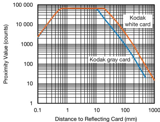
Fig. 12 - Proximity Value vs. Distance for 8T and 200 mA
