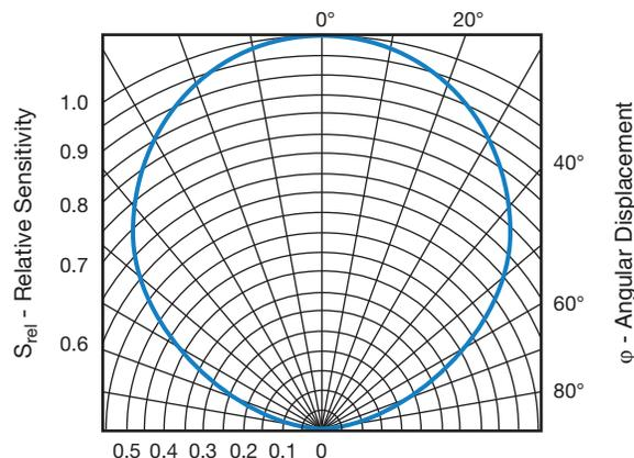
Fig. 5 - Angle of Half Sensitivity of the Photodiode
