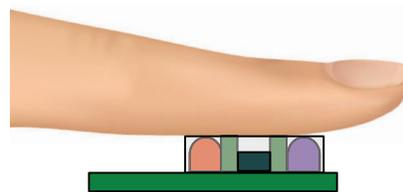
Fig. 34 - Sensing in Reflective Mode With the VCNL3036
