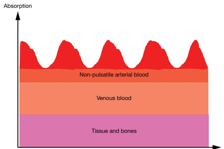
Fig. 36 - Heart Rate Pulsing and Other Reflected Light
