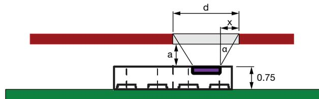
Fig. 8 - Window Dimensions for One Hole (in millimeters)
