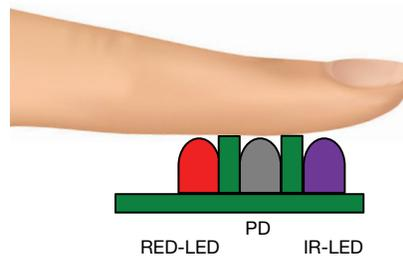
Fig. 33 - Sensing in Reflective Mode
