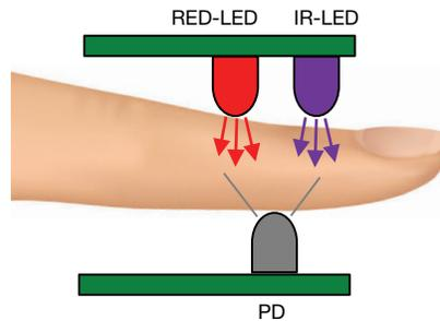
Fig. 32 - Sensing in Transmissive Mode
