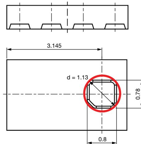
Fig. 7 - Light Hole Diameter (in millimeters)
