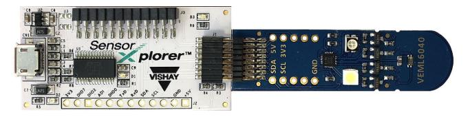
After having connected the sensor board to the SensorXplorer and the SensorXplorer to the PC, unzip the respective demo software. Open the unzipped folder and start the executable from within the folder:
