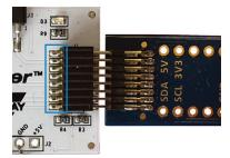
The pinning of the connector is mirrored on the SensorXplorer board, so there is an option of connecting the board the other way around; however, this is not recommended, as the connector has pins on the SensorXplorer board side of the connector, as indicated above. If the sensor board is connected the other way around, care must be taken not to push the sensor board all the way through, as this will lead to a short circuit.
