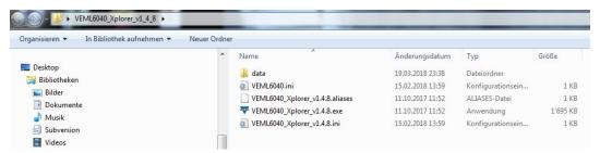
The data folder contains the required DLLs for the executable to run and for the hardware communication to function. This folder should not be moved or deleted, as the executable references it as a relative path.
