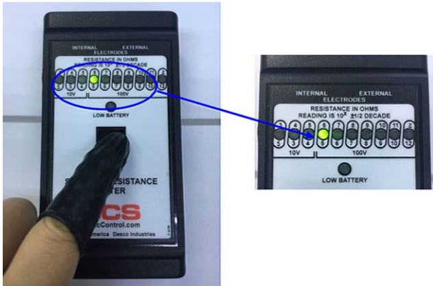
Fig. 4 - Typical Surface Resistance Values of the Cover Tape
