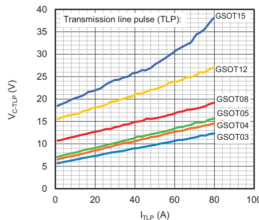
Fig. 6 - Typical Clamping Voltage vs. Peak Pulse Current
