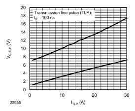
Fig. 5 - Typical Clamping Voltage vs. Peak Pulse Current
