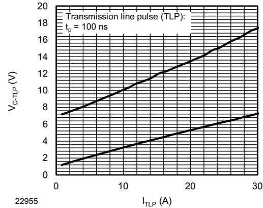
Fig. 5 - Typical Clamping Voltage vs. Peak Pulse Current
