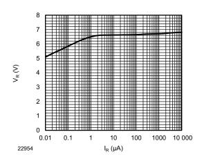
Fig. 4 - Typical Reverse Voltage vs. Reverse Current
