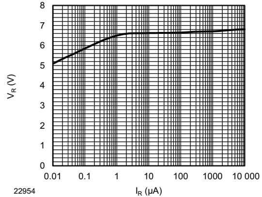
Fig. 4 - Typical Reverse Voltage vs. Reverse Current
