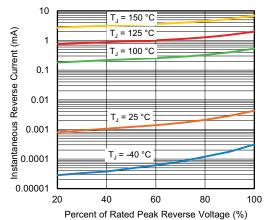
Fig. 4 - Typical Reverse Characteristics
