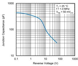
Fig. 5 - Typical Junction Capacitance
