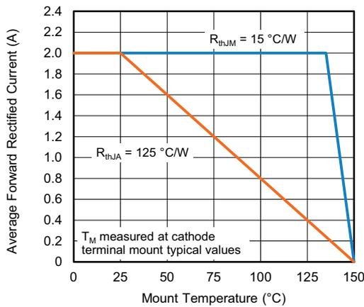
Fig. 1 - Maximum Forward Current Derating Curve
