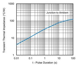
Fig. 6 - Typical Transient Thermal Impedance
