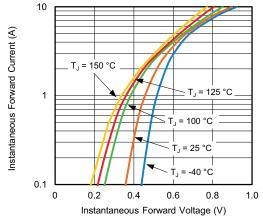
Fig. 3 - Typical Instantaneous Forward Characteristics
