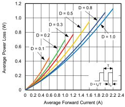
Fig. 2 - Forward Power Loss Characteristics
