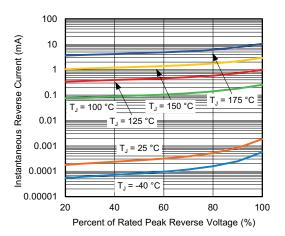
Fig. 4 - Typical Reverse Characteristics
