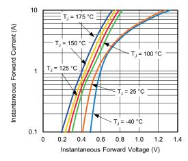
Fig. 3 - Typical Instantaneous Forward Characteristics
