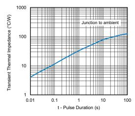
Fig. 6 - Typical Transient Thermal Impedance
