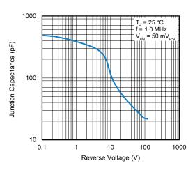
Fig. 5 - Typical Junction Capacitance
