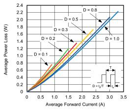
Fig. 2 - Forward Power Loss Characteristics
