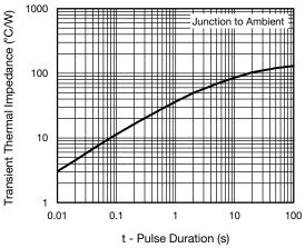
Fig. 6 - Typical Transient Thermal Impedance
