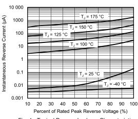
Fig. 4 - Typical Reverse Leakage Characteristics
