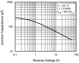
Fig. 5 - Typical Junction Capacitance
