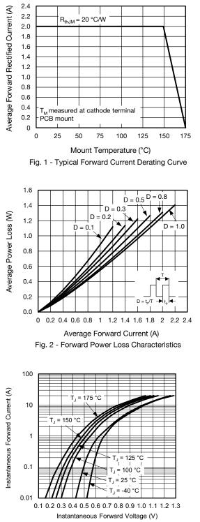
Fig. 3 - Typical Instantaneous Forward Characteristics
