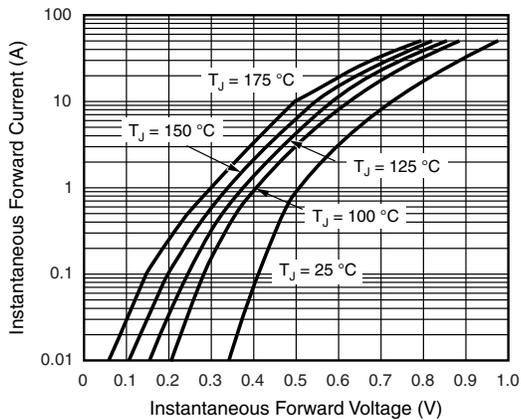
Fig. 3 - Typical Instantaneous Forward Characteristics Per Diode
