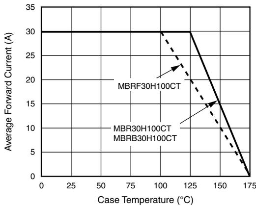
Fig. 1 - Forward Derating Curve Per Diode
