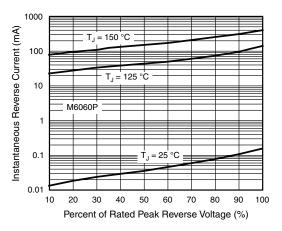
Fig. 8 - Typical Reverse Characteristics Per Diode
