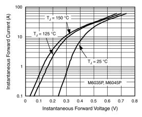
Fig. 5 - Typical Instantaneous Forward Characteristics Per Diode
