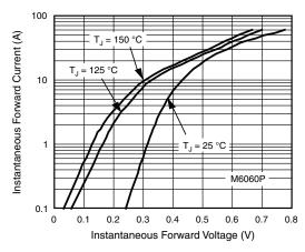
Fig. 6 - Typical Instantaneous Forward Characteristics Per Diode
