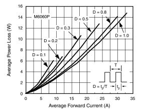
Fig. 3 - Forward Power Loss Characteristics Per Diode
