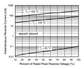
Fig. 7 - Typical Reverse Characteristics Per Diode
