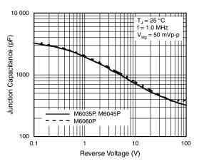
Fig. 9 - Typical Junction Capacitance Per Diode
