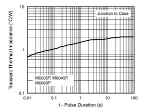
Fig. 10 - Typical Transient Thermal Impedance Per Diode
