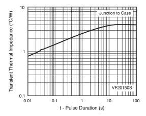
Fig. 7 - Typical Transient Thermal Impedance
