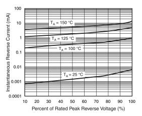
Fig. 4 - Typical Reverse Characteristics
