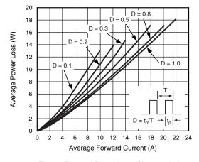
Fig. 2 - Forward Power Loss Characteristics
