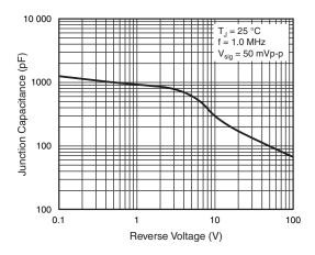
Fig. 5 - Typical Junction Capacitance
