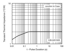
Fig. 6 - Typical Transient Thermal Impedance
