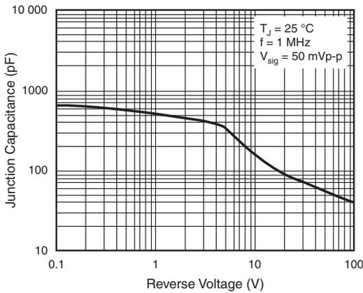
Fig. 6 - Typical Junction Capacitance Per Diode
