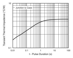
Fig. 7 - Typical Transient Thermal Impedance Per Diode
