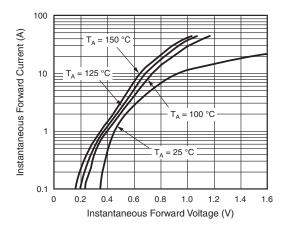
Fig. 4 - Typical Instantaneous Forward Characteristics Per Diode
