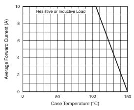
Fig. 1 - Forward Current Derating Curve
