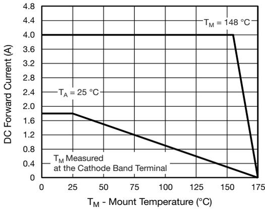
Fig. 1 - Maximum DC Forward Current Derating Curve
