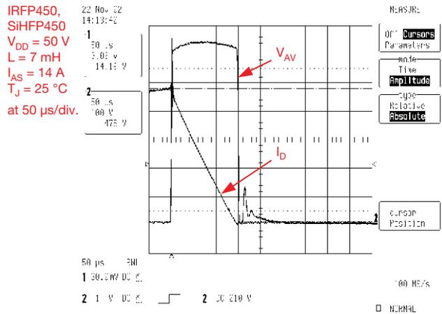
Fig. 16 - IRFP450, SiHFP450 (500 V Rated) Device Avalanche Waveforms
