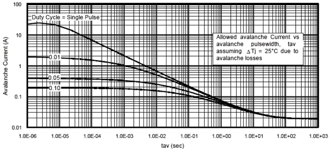
Fig. 21 - Typical Avalanche Current vs. Pulsewidth For Various Duty Cycles
