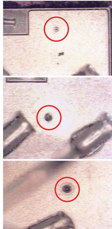
Fig. 8 - Power MOSFET Random Device Failure Spots
