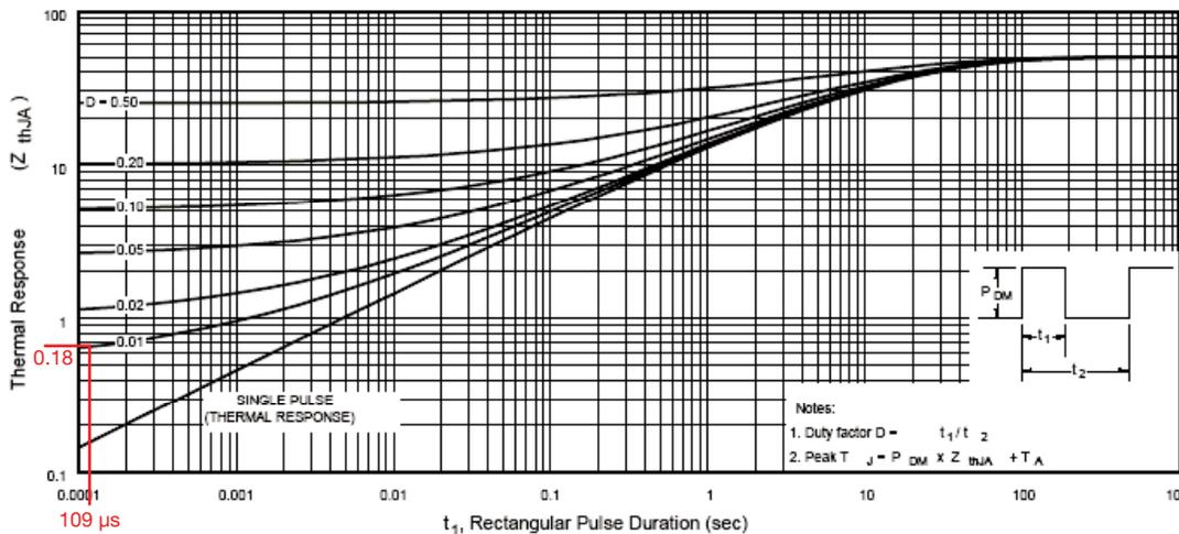
Fig. 23 - Typical Effective Transient Thermal Impedance, Junction-to-Ambient
