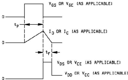
Fig. 12 - Single Pulse Unclamped Inductive Switching Test Circuit Output Waveforms
