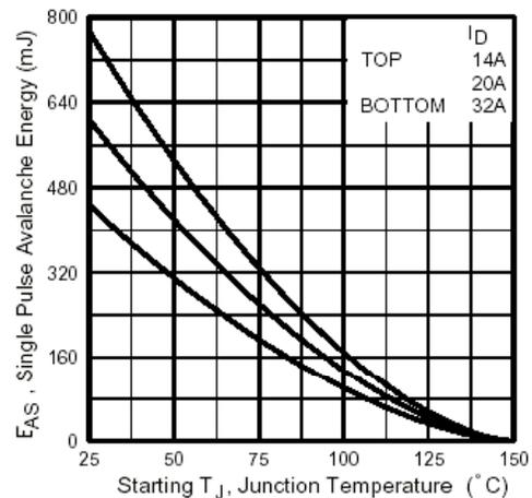
Fig. 19 - Maximum Avalanche Energy vs. Temperature For Various Drain Currents
