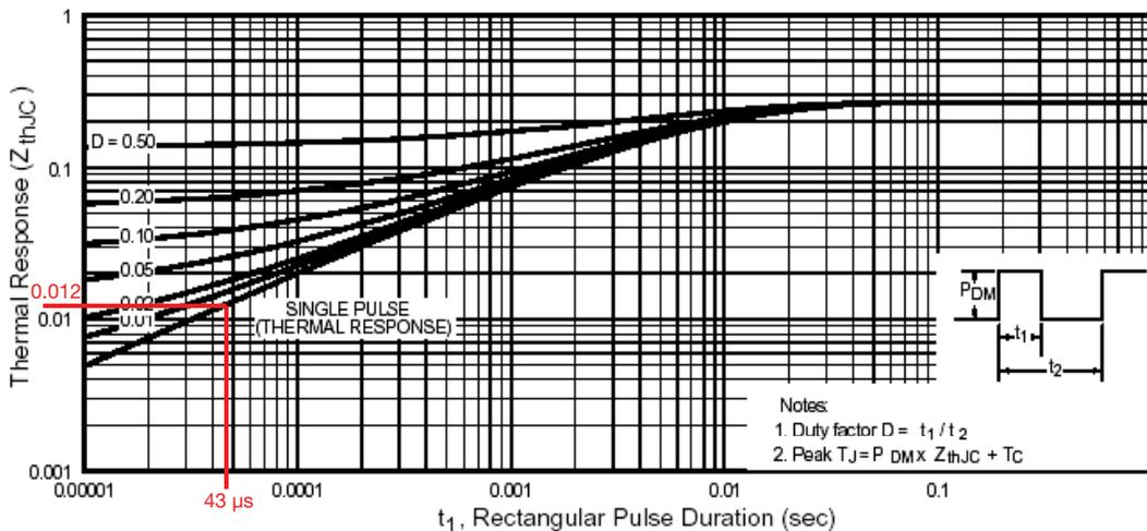
Fig. 18 - Transient Thermal Impedance Plot, Junction-to-Case
