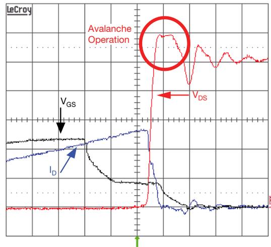
Fig. 3 - Flyback Converter Switch Under Avalanche Waveform (Detail)
