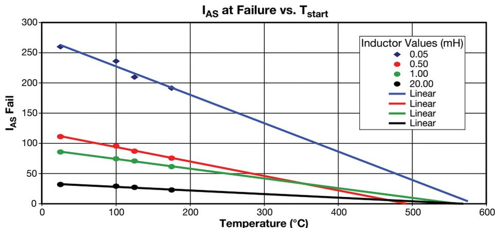
Fig. 10 -  $I_{AS}$  at Failure vs. Test Temperature
