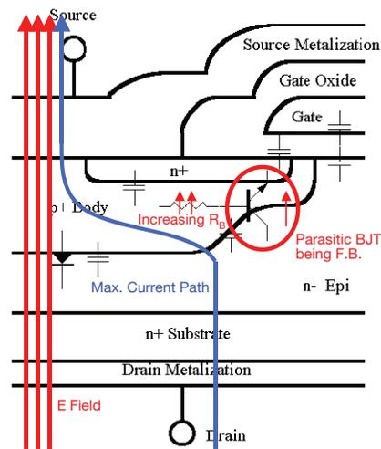
Fig. 6 - Power MOSFET Cross Section Under Avalanche
