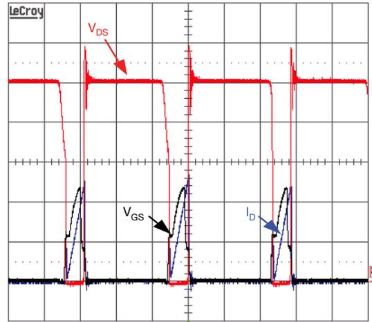
Fig. 2 - Flyback Converter Switch Under Avalanche Waveform
