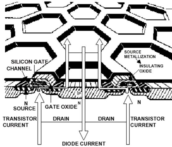
Fig. 7 - Basic Power MOSFET Cell Structure
