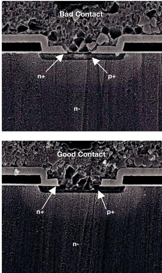
Fig. 9 - Good Source Contact vs. Bad Source Contact Illustration
