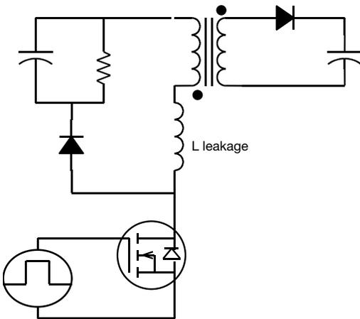
Fig. 1 - Flyback Converter Circuit
