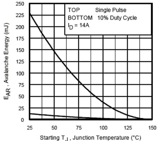
Fig. 20 -  $E_{AR}$  vs.  $T_{start}$  For Various Duty Cycles, Single  $I_D$
