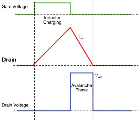
Fig. 15 - Typical Simulated Avalanche Waveforms
