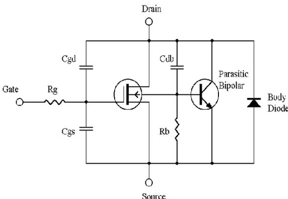
Fig. 5 - Power MOSFET Circuit Model
