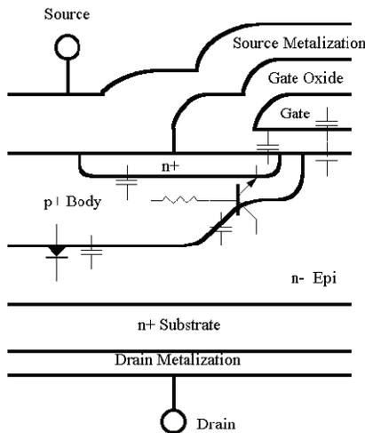
Fig. 4 - Power MOSFET Cross Section
