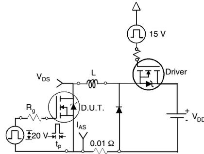
Fig. 13 - Decoupled  $V_{DD}$  Voltage Source Test Circuit Model
