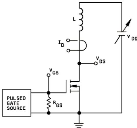
Fig. 11 - Single Pulse Unclamped Inductive Switching Test Circuit
