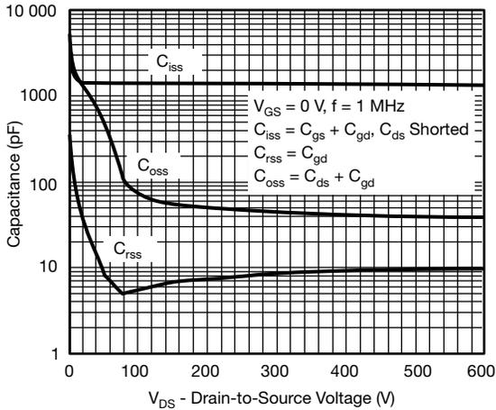
Fig. 3a) Super Junction Technology Capacitive Plot
