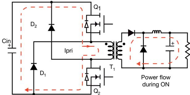
Fig. 1a) Power Transfer Stage of Operation
