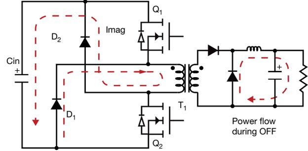
Fig. 1b) Power Flow from Output Cap to Power Load
