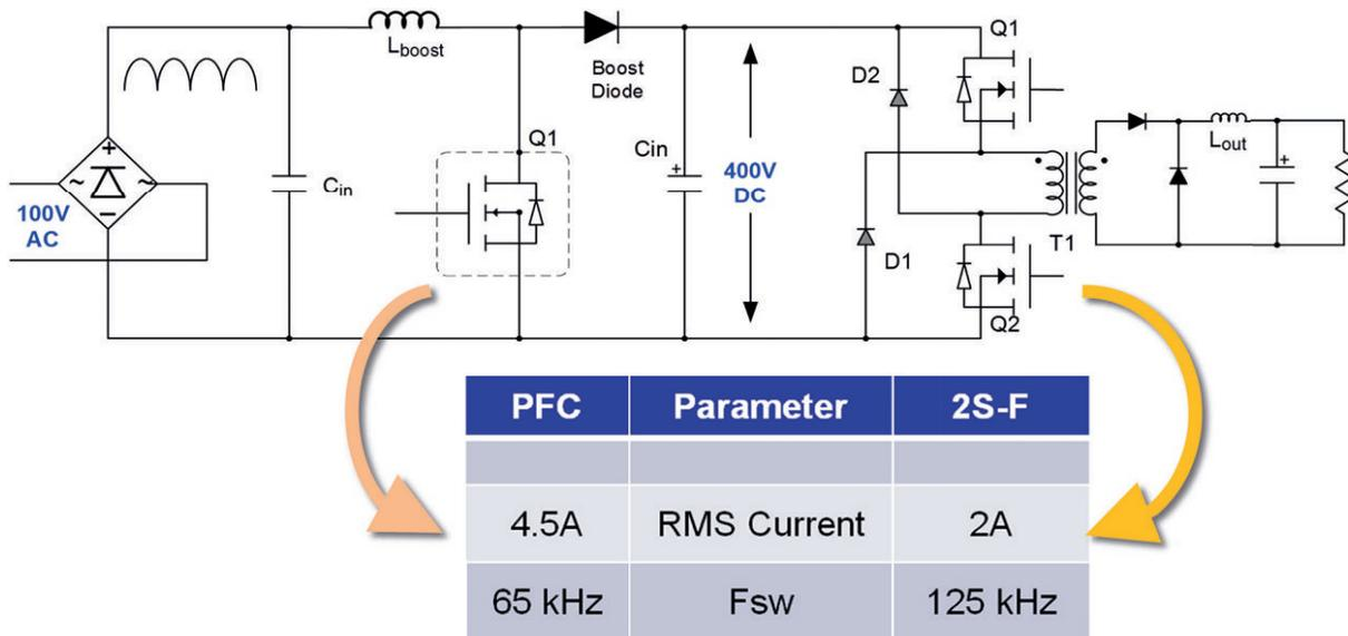
Fig. 2 Power Factor Correction Converter vs. a Two-Switch Forward Converter
