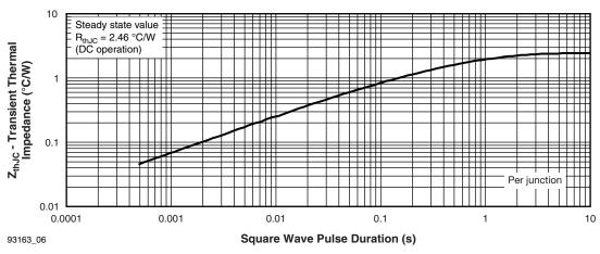
Fig. 6 - Thermal Impedance ZthJC Characteristics
