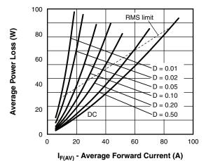
Fig. 6 - Forward Power Loss Characteristics
