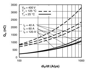
Fig. 8 - Typical Stored Charge vs. di<sub>F</sub>/dt
