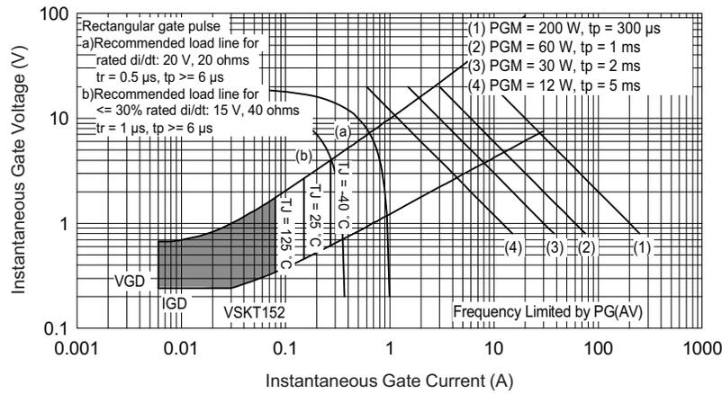
Fig. 12 - Gate Characteristics
