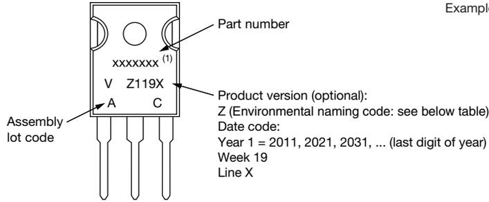
Example: This is a xxxxxxx<sup>(1)</sup> with assembly lot code AC, assembled on WW 19, 2021 in the assembly line "X"
