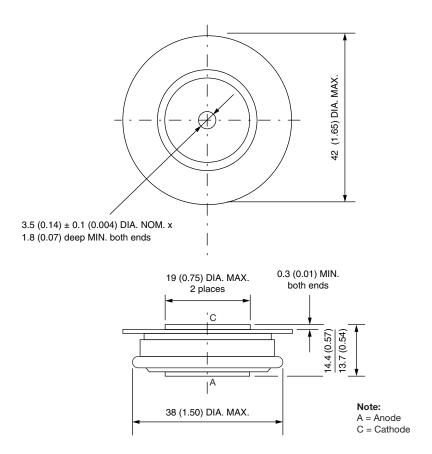
Quote between upper and lower pole pieces has to be considered after application of mounting force (see Thermal and Mechanical Specifications)
