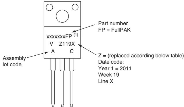
Example: This is a xxxxxxxFP<sup>(1)</sup> with assembly lot code AC, assembled on WW 19, 2011 in the assembly line "X"
