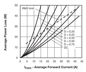
Fig. 7 - Forward Power Loss Characteristics
