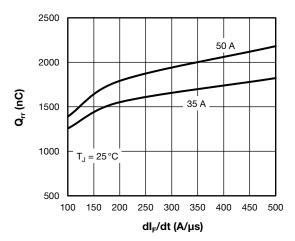
Fig. 9 - Typical Stored Charge vs.  $dI_F/dt$
