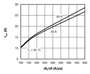
Fig. 11 - Typical Reverse Current vs. dl<sub>F</sub>/dt
