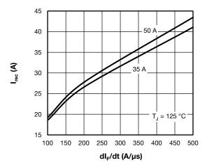
Fig. 12 - Typical Reverse Current vs. dl<sub>F</sub>/dt
