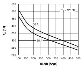
Fig. 8 - Typical Reverse Recovery Time vs. dl<sub>F</sub>/dt
