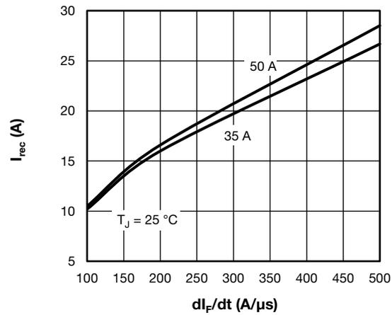
Fig. 11 - Typical Reverse Current vs.  $dI_F/dt$
