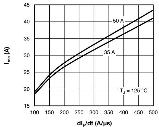
Fig. 12 - Typical Reverse Current vs.  $dI_F/dt$
