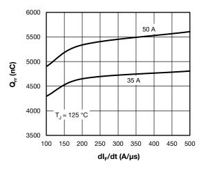
Fig. 10 - Typical Stored Charge vs. dl<sub>F</sub>/dt
