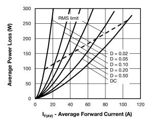
Fig. 6 - Forward Power Loss Characteristics
