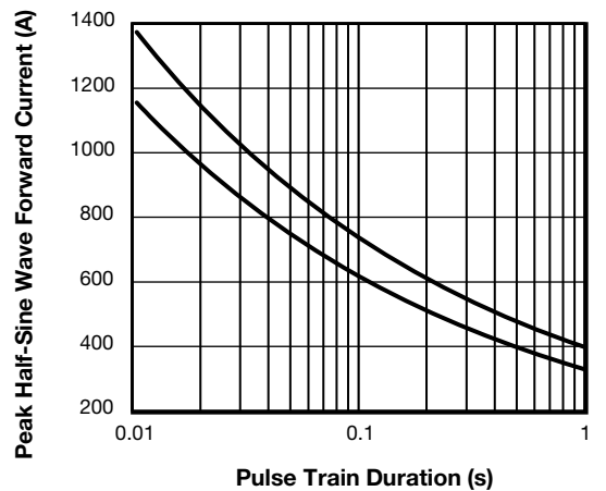
Fig. 6 - Maximum Non-Repetitive Surge Current
