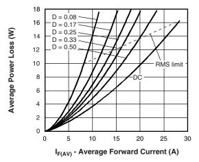
Fig. 6 - Forward Power Loss Characteristics
