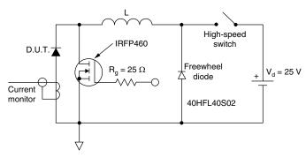
Fig. 8 - Unclamped Inductive Test Circuit
